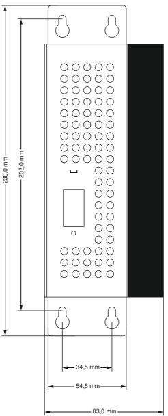
The device may only be installed in a vertical position, with the connection side at the bottom.
