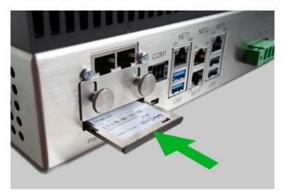
**Attention:** The CFast card may only be inserted in the way described here without significant effort! Forcible, twisted or tilted insertion will damage the CFast socket!
