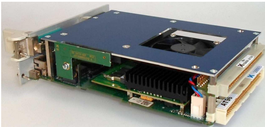
H1/103 version with „Rear-Extender“ and carrier plate for 2,5“-SATA-SSD.
